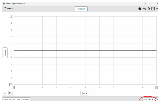
Figure 1: The red oval indicates where to click to calibrate the force sensor.
